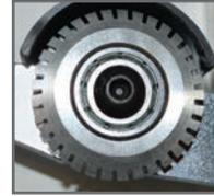
The perf wheel that comes standard with all COUNT™ machines has 33 teeth, or 9 cuts per inch.
